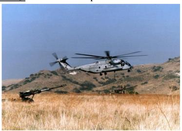
The heavy-lift helicopter of the Marine Corps can carry a 26,000-pound Light Armored Vehicle, 16 tons of cargo 50 miles and back, or enough combat-loaded Marines to lead an assault or humanitarian operation.
